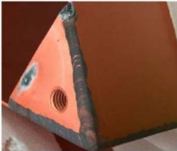
ANODISED ALUMINIUM COMPONENT MANUFACTURED WITH 4043 / 4047 TIG ROD (BLACK FINISH ON WELD)
