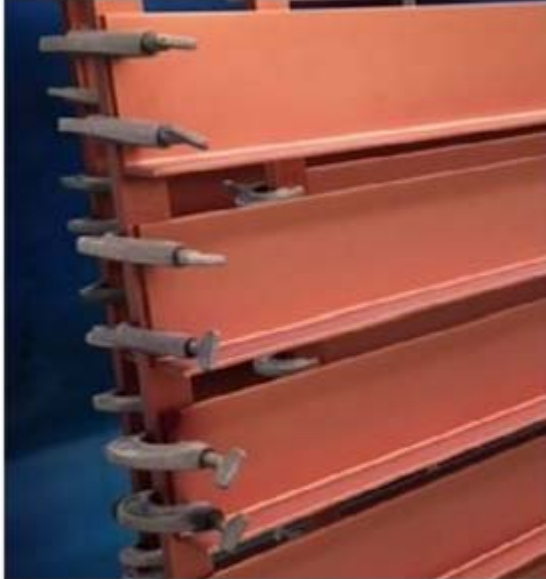
CLAMP MARK ON EXTRUSION UP TO 50MM WILL HAVE A CONTACT MARK ON BACK AND IS WASTE, FRONT WILL HAVE ROUND MARK FROM CLAMP SCREW
